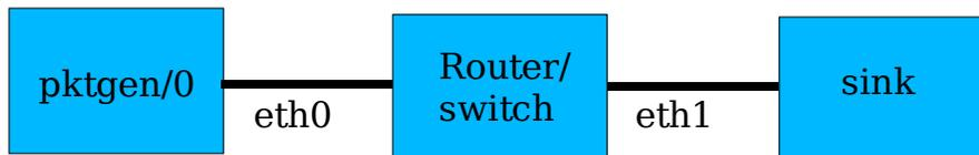
Forwarding setup using dual devices. Pktgen can use different threads to achieve high load in terms of small packets or concurrent flows.
